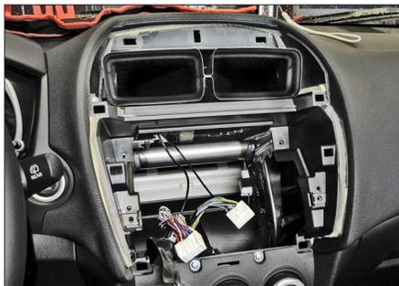
3. Dashboard with removed OEM Radio/CD device
